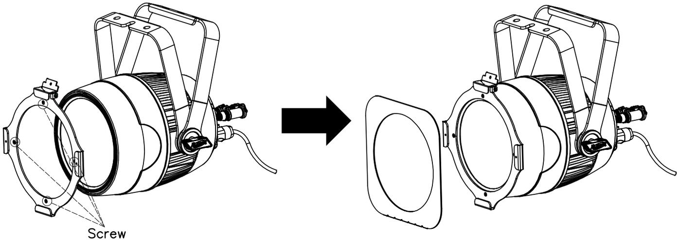
1. Remove BARN DOOR / GEL FRAME HOLDER from shipping box and separate.
