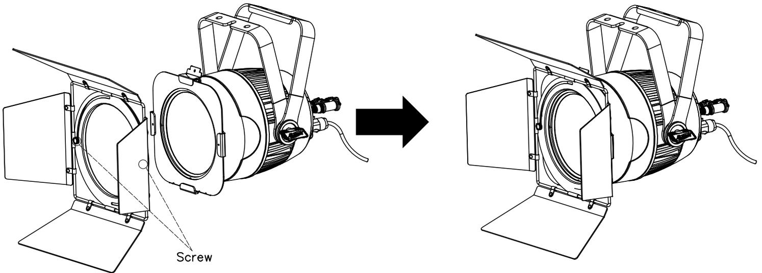
4. Push back retention clip and slide BARN DOOR down into GEL FRAME HOLDER.
