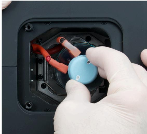
9. Install and position lamp so it is seated properly, then secure retention clip. (See below)
