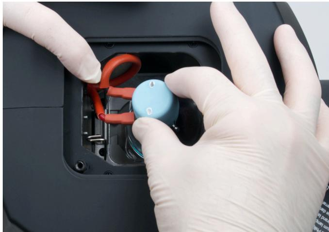
4. Gently remove **(2) Wires** connected to spade terminals on lamp. (See below)
