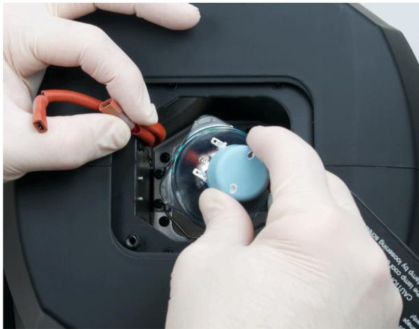
7. Gently attach **(2) Wires** to spade terminals on the base of the lamp. (See below)
