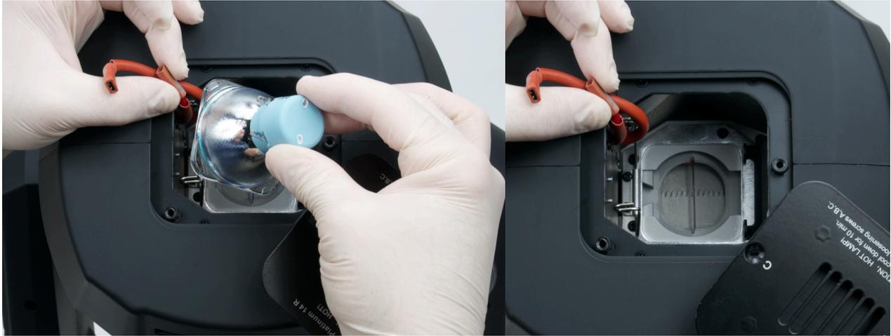
6. Using thumb and index finger, gently install new lamp into the fixture. (See below)
