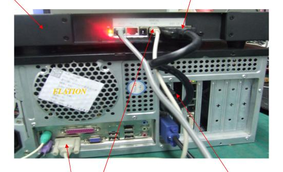
Connect the RS232 data cable into your PC (Use the RS232 to USB convertor if you don't have RS232 on your PC). Connect RJ11 end into the EVLED-VSC.
