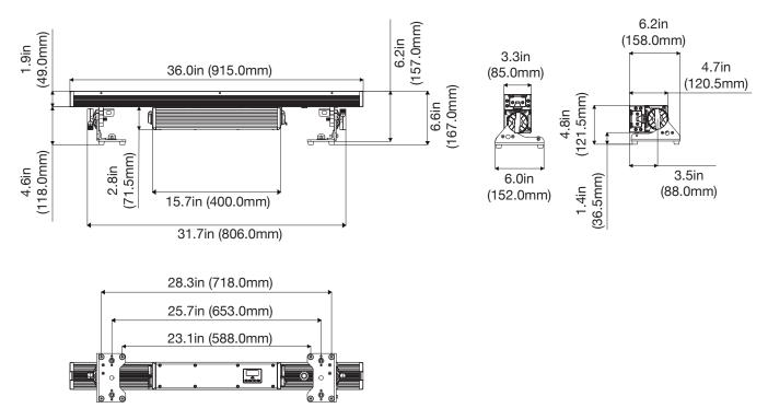
GLARE SHIELD INSTALLED (same as above unless otherwise stated)
