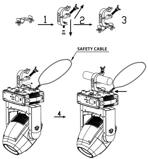
Screw one clamp each via a M12 screw and nut into the Omega bracket. Insert the quick-lock fasteners of the Omega holder's into the respective holes on the bottom of the Focus Spot 4Z/Focus Spot 4Z Pearl. Tighten the quick-lock fasteners fully clockwise. Pull the safety cable through the openings located on the base plate and over the trussing system or a safe fixation spot. Insert the end in the carabine and tighten the safety screw.
