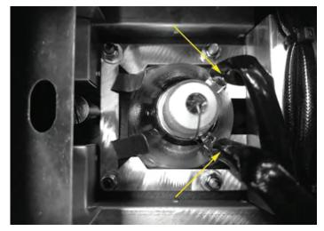
3. Gently remove the (2) spade terminals connected to the lamp.
