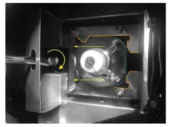
4. Use a flat head screwdriver to turn the lamp centering screw clockwise until the lamp slides out of its holder on the right side.
