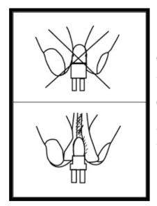
This fixture is fitted with a DISCHARGE LAMP, which is highly susceptible to damage if improperly handled. NEVER touch the lamp with your bare hands, as the oil from your hands will shorten the life of the lamp. NEVER move the fixture until the lamp has had ample time to cool. Lamps are NOT covered under warranty conditions. Avoid switching the fixture ON and OFF repeatedly in short intervals, as this will reduce lamp life and intensity.
