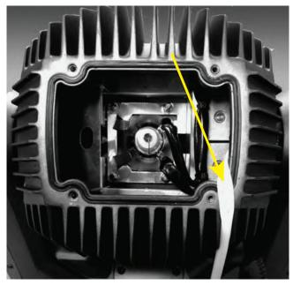
2. Unscrew the (4x) allen head screws, then remove the rear cover. Please be advised that the cover is connected to the unit via a safety cable and connected wire cable.
