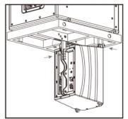
3. Position **IMPERIO** speaker underneath **Imperio Flybar LG** & secure front holes with **Linkpin 1** locking-pins, and bracket with **Linkpin 2** locking-pins.
