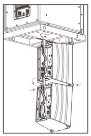
4. Hang second **IMPERIO** speaker and secure front holes with **Linkpin 1** locking-pins & adjust throw bracket by select desired throw angle, and secure with **Linkpin 2** locking-pins.
