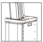
3. Position IMPERIO PRO speaker on Imperio Flybar LG and secure front holes with Linkpin 1 locking-pins.
