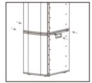
1. With 2X stacked **Subs**, secure 2. Locate **Imperio Flybar LG** them with **Linkpin 1** locking- on top stacked sub and pins, and connect with power and XLR cables.
