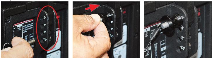
Adjust throw angle by attaching integrated adjustable mounting bracket from IMPERIO spéaker, swinging it down to desired throw angle mounting hole on bottom IMPERIO speaker or Flybar, secure with Linkpin 2.
