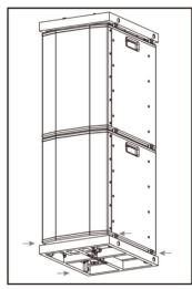
2. Secure **Imperio Sub Flybar** underneath bottom (hanging) sub & secure with **Linkpin 2** locking-pins.
