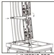
5. Stack second **IMPERIO PRO** speaker, secure front holes with Linkpin 1 locking-pins, then select desired throw angle and secure with Linkpin 2 locking-pin.
