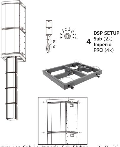
1. Secure top **Sub** to **Imperio Sub Flybar** with **Linkpin 2** locking-pins, then secure second hanging **Sub** with **Linkpin 1** locking-pins.
