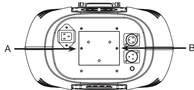
**Optimizing Lamp Alignment:** This procedure centers the lamp in the reflector. Proper optimization will increase lamp life and ensure a bright crisp output. Improper optimization may add a yellow tint to the lamp output and reduce intensity.
