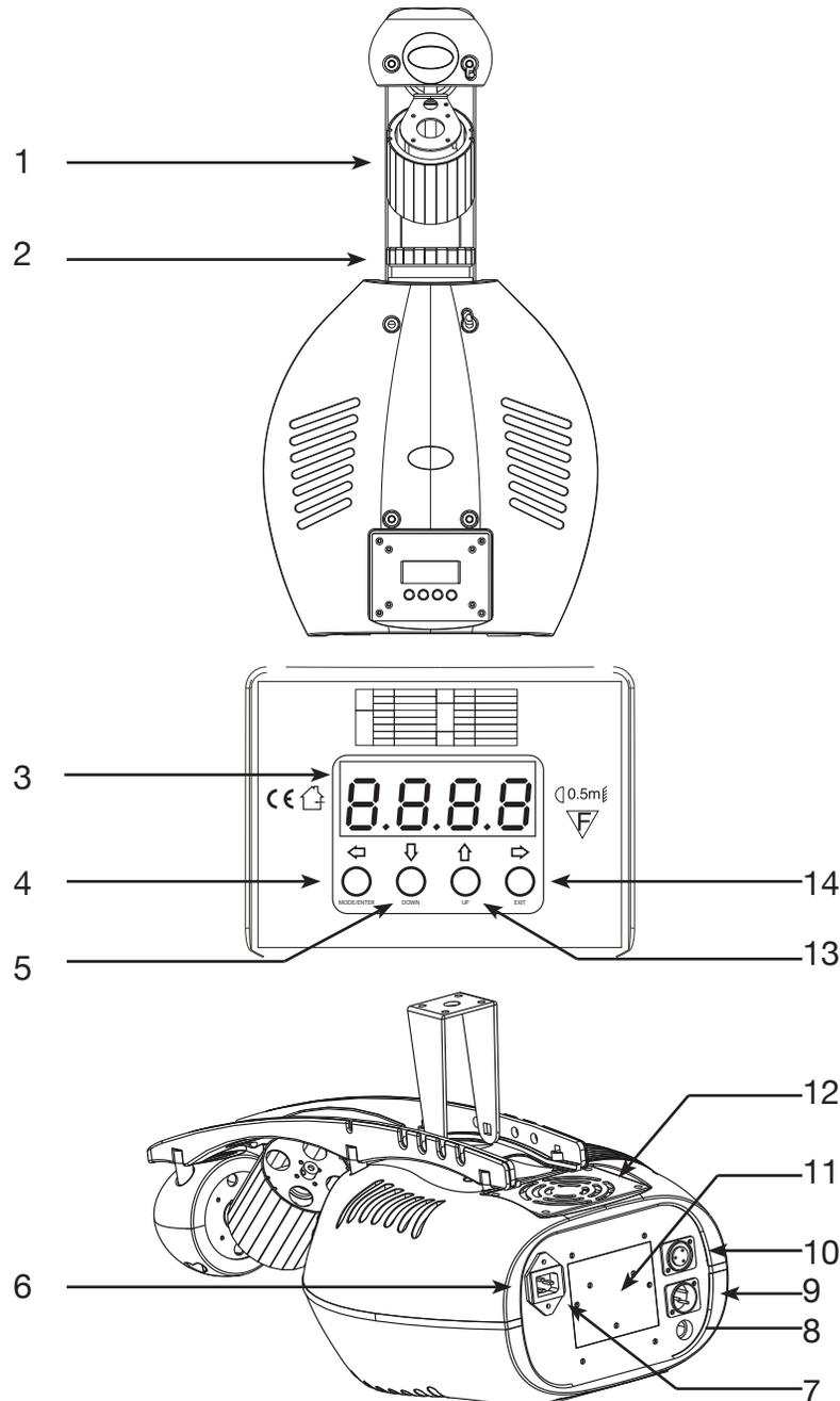
**1. Barrel Mirror** - This is a highly reflective surface mirror specifically designed to optimize and enhance beam output. Never use glass cleaner that contain ammonia to clean the surface of the mirror (such as Windex).
