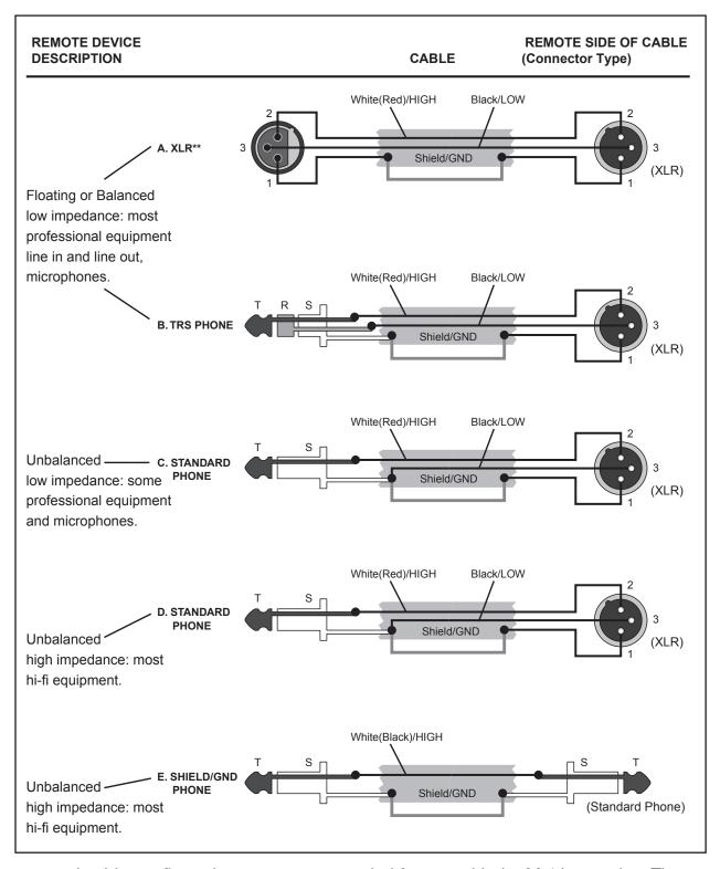
Connector and cable configurations are recommended for use with the M 4 bus series. These cables are based on the use of auxillary equipment that is isolated from the AC power mains.
