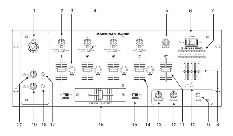
**1. MICROPHONE 1** - This combo jack will accept a standard 1/4 plug or XLR 3-pin balanced male plug. The volume output level for this microphone will be controlled by its own respective CHANNEL KNOB (20). Note: We recommend that you use a 500-600ohm microphone for the best sound quality.
