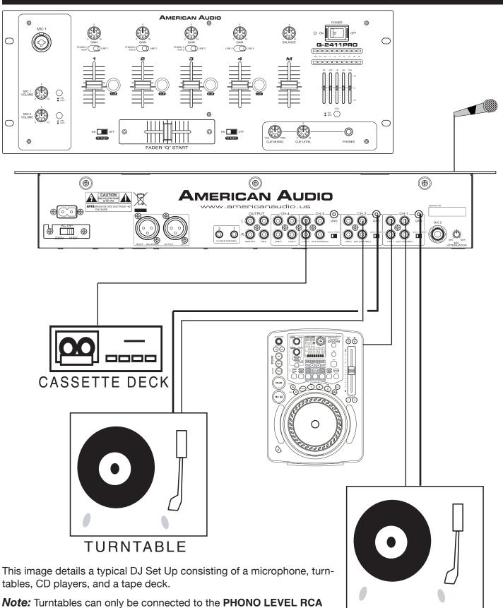
**Note:** Turntables can only be connected to the **PHONO LEVEL RCA JACKS**. Be sure the **LINE LEVEL SELECTOR SWITCHES** are in the "PHONO" position when using turntables.
