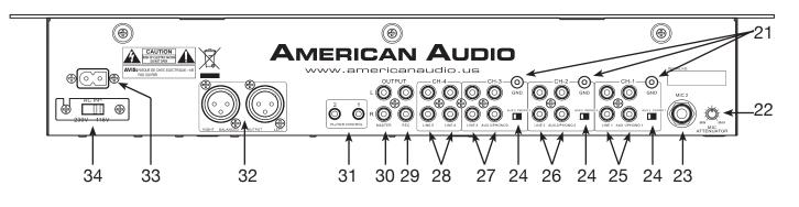
**21. GND (GROUND TERMINAL)** - Be sure to connect turntable ground leads to either or both of the two available ground terminals. This will reduce the humming and popping noises associated with magnetic phono cartridges.
