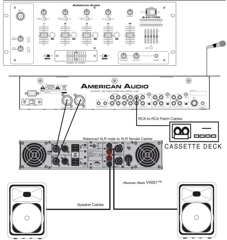
Typical Balanced Output Set-up
