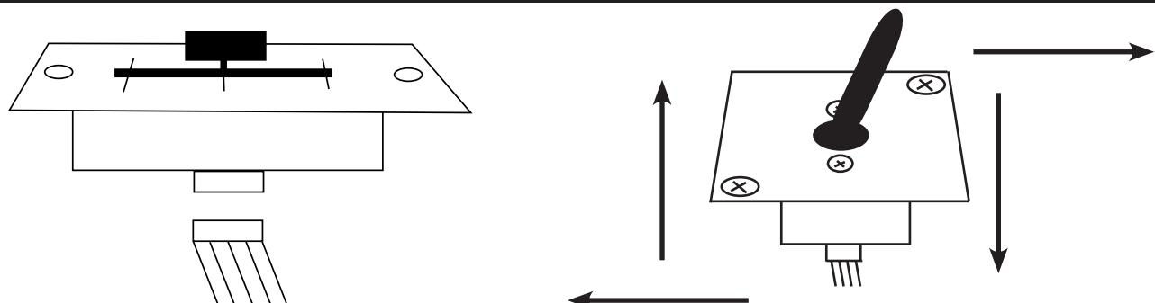
*The crossfader is "Hot Swappable" which means it may be replaced at any time, even when power is applied. Only replace with American Audio Part OF-1. Replacing with any other model fader may seriously damage your mixer.*
