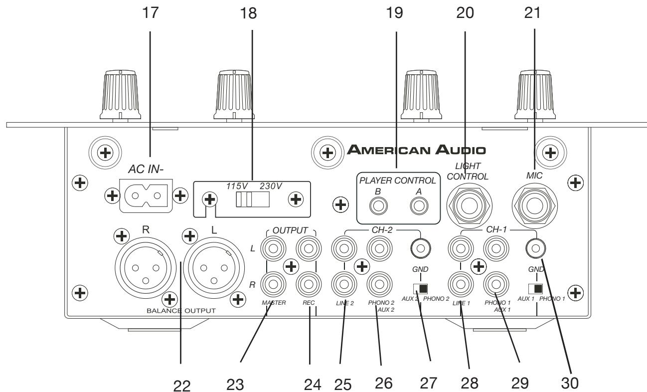
**17. AC CONNECTION** - This connector is used to supply main power to the unit via the included detachable power cord. Use only the supplied, polarized AC power cord. This cord is designed to fit in one direction only. Do not attempt to force a cord in if it does not fit, be sure the cord is being inserted properly
