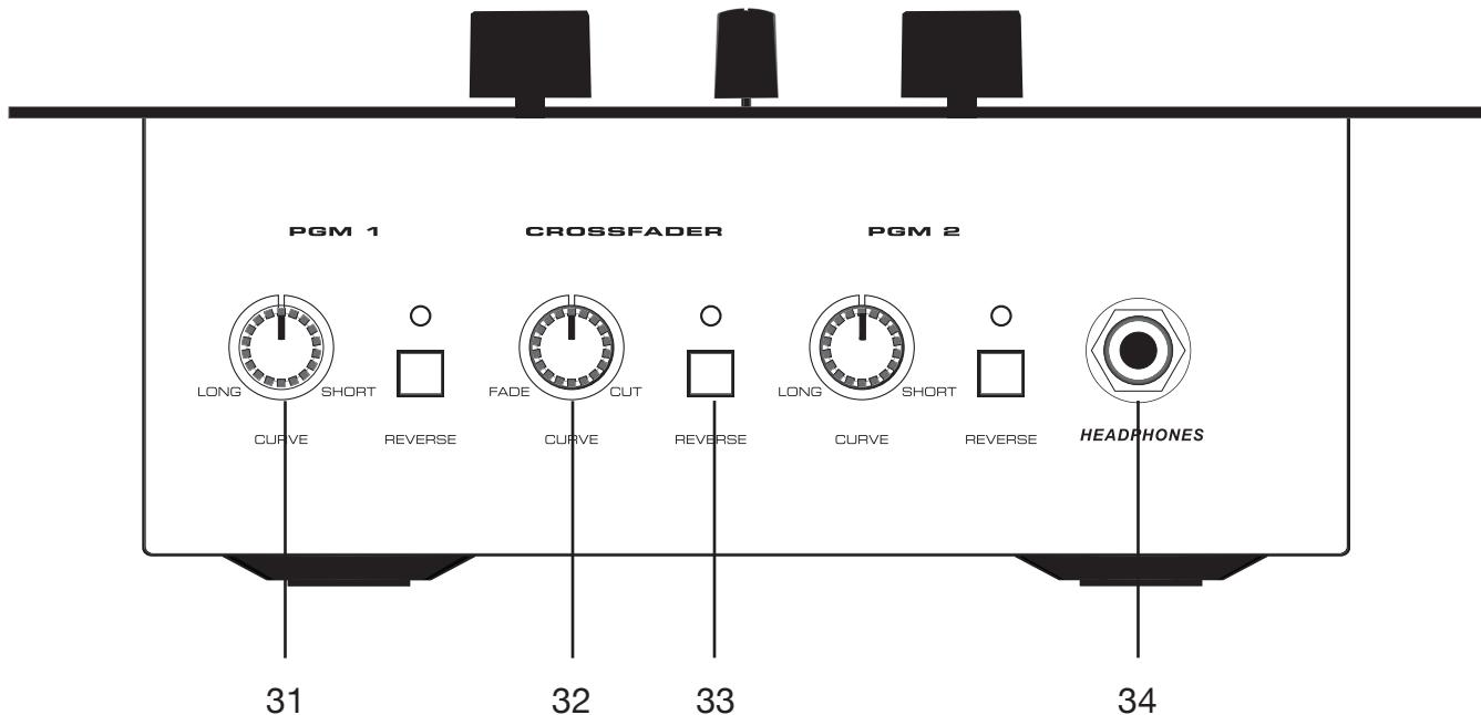
**31. CHANNEL FADER CURVE ADJUSTMENT** - This rotary knob is used to change the way the channel fader will operate. Each of the two channels has a “Curve” adjustment. The curve on the faders adjust from long or short or any variation of the two. The shorter the curve adjustment the sooner full volume will be reached.
