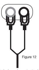
Typical speaker output using spade connectors. Insert bare wire into the binding post and tighten.
