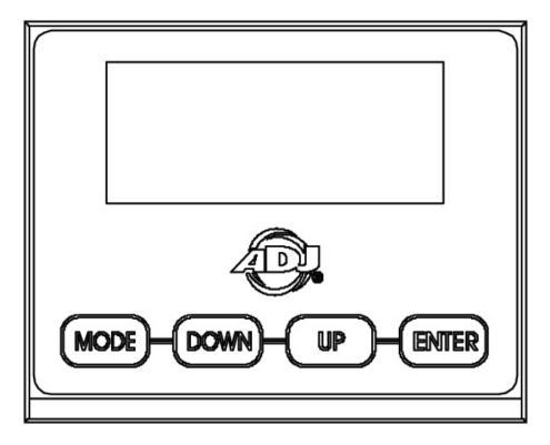
This device features two different settings for locking the keypad. Setting Lock to "ON" requires the user to simply press and hold the MODE button for 10 seconds to unlock the keypad.
