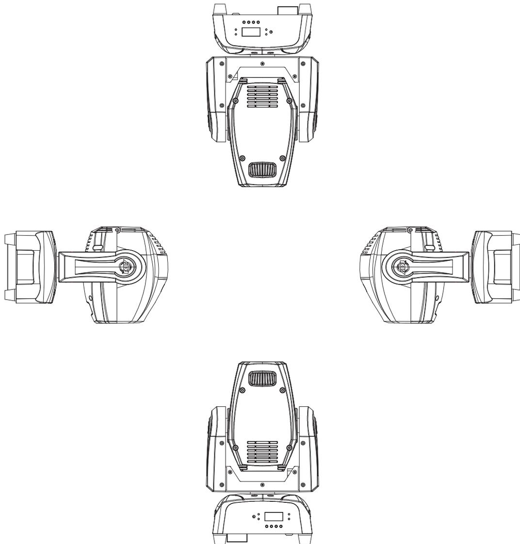
The Focus Spot 2X is fully operational in three different mounting positions, hanging upside-down from a ceiling or trussing, sideways on trussing, or set on a flat level surface. Be sure this fixture is kept at least 12m (40ft) away from any flammable materials (decoration etc.). Always use and install the supplied safety cable as a safety measure to prevent accidental damage and/or injury in the event the clamp fails (see next page). Never use the carrying handles for secondary attachment.
