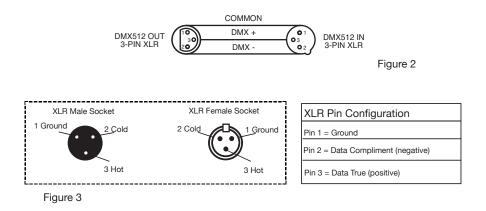
**Special Note: Line Termination.** When longer runs of cable are used, you may need to use a terminator on the last unit to avoid erratic behavior. A terminator is a 110-120 ohm 1/4 watt resistor which is connected between pins 2 and 3 of a male XLR connector (DATA + and DATA -). This unit is inserted in the female XLR connector of the last unit in your daisy chain to terminate the line. Using a cable terminator (ADJ part number Z-DMX/T) will decrease the possibilities of erratic behavior.
