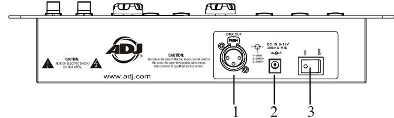
1. DMX OUT - Used to send DMX signal to the compatible LED fixtures.
