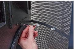
3. Slip your hand in between the grille and speaker and disconnect the Clip LED wire.
