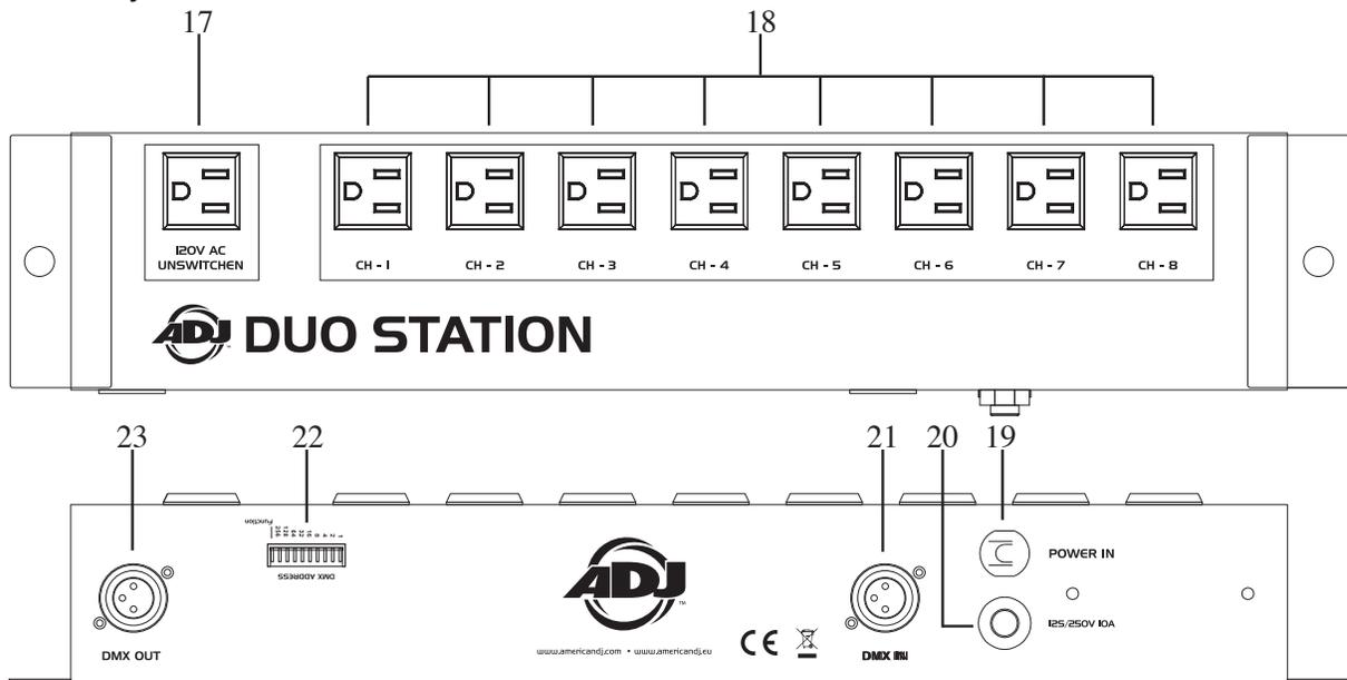
17. 120V AC “CONSTANT” POWER SOCKET - This is the main power socket. This socket will always have power regardless of the dipswitches.
