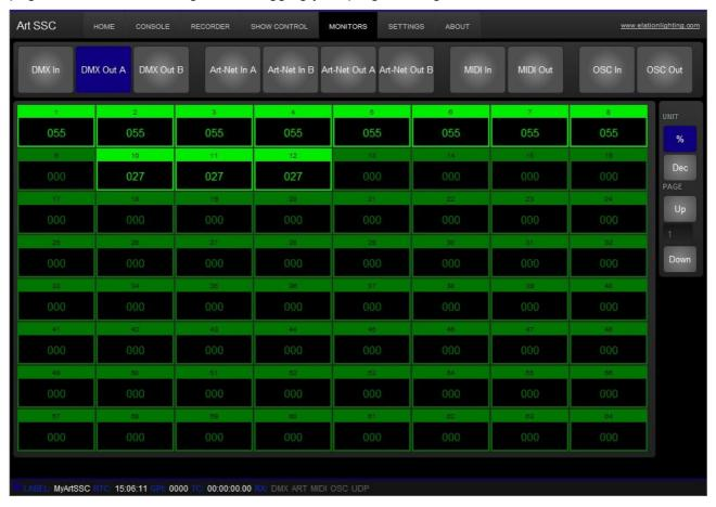
The top row of buttons allows for selecting the data stream. In the case of DMX or Art-Net data, you can use the buttons on the right to toggle between decimal and percentage notations, and use the up and down buttons to step through all the channel pages.
