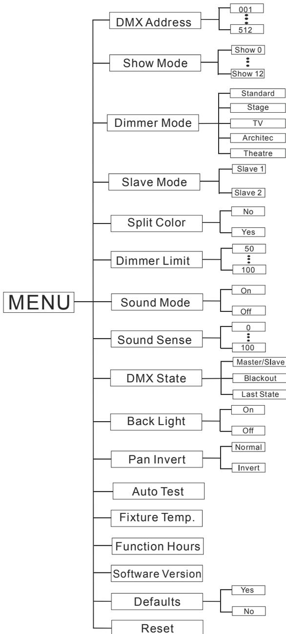
**System Menu:** When making adjustments press ENTER to confirm your setup then press and hold the MENU button for at least 3 seconds. To exit without making any adjustments press the MENU button. The display will lock after 30 seconds, press the MENU button for 3 seconds to unlock.
