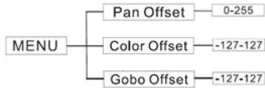
To enter the offset adjustment submenu, press the ENTER button for at least 5 seconds. In this submenu you are able to adjust the original position of the pan, gobo wheel, and color wheel.
