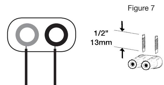
Typical speaker output using bare wire. Insert bare wire into the binding post and tighten.
